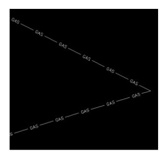
Notice the text is now upright in both segments. Using the U in the linetype definition sets the "Upright" flag. Setting it to 0.0 keeps it Upright relative to the line. I played around with it a bit and, unfortunately, it doesn't seem to help much when rotating with DVIEW or UCS. But, when you're working in world coordinates, this is a great tool.
