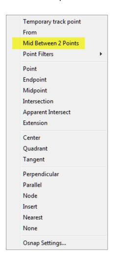
Next you'll be prompted to specify two new points for which you can use additional OSnap settings. The example below shows a new line that starts at the Midpoint between the ENDpoints of the two existing lines.
