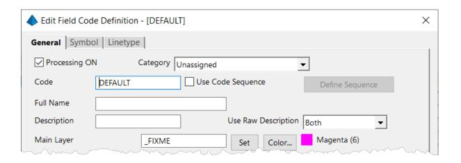
This is a "slightly known" feature that's built into Carlson Software's Field to Finish feature. The Field to Finish command is available in the Carlson Survey, Construction and Takeoff programs. Please see the video below to learn how to use the DEFAULT field code to quickly identify and find points with random, non-standard, descriptions that may need your attention.
