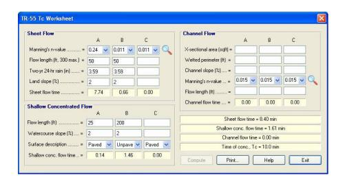
There is a 5.1 minute difference in TC results which results in a 2 CFS difference in the 100yr example below:
