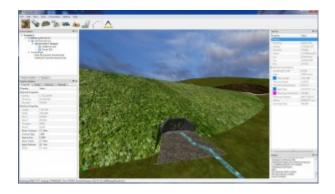
Once a digital terrain model from CAD, Google Earth, or other source is imported, the on-screen image accurately reflects the materials represented, such as roadways, embankments, rocks, fields, etc.
