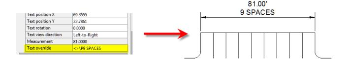
And, finally, one more option. Rather than entering "P", if you enter "X" as part of your Text override, you will stack the text partially above and partially below the dimension line.
