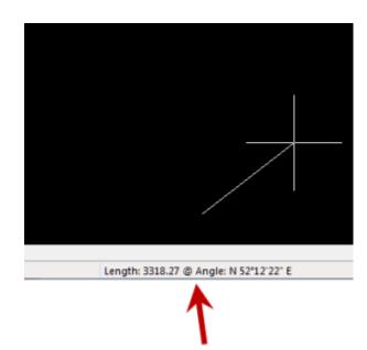
To toggle the coordinate display in newer versions of AutoCAD (since 2009?) double-click on the coordinate display. In older
